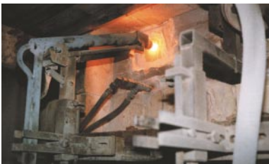
Oxygen Lancing – Detail
